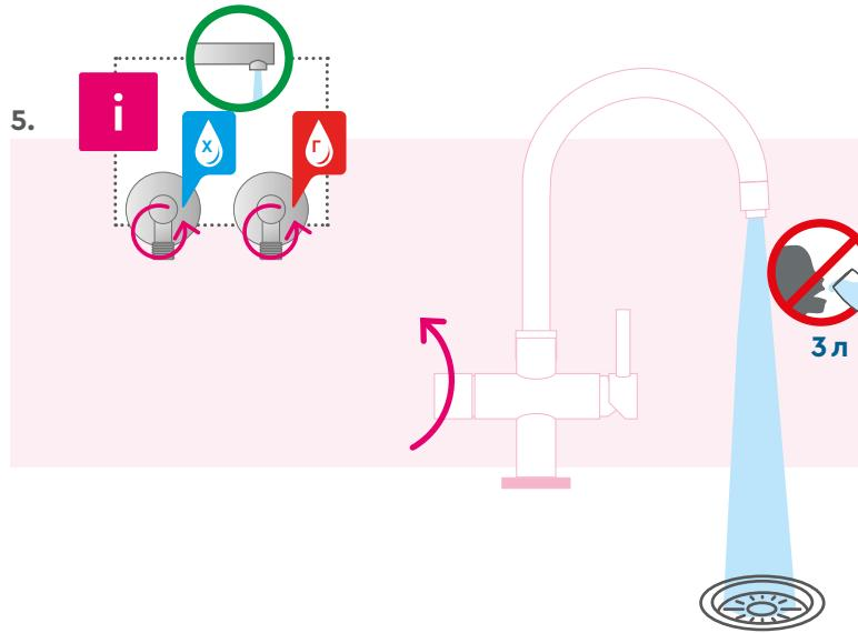
**DE** Flush the filter cartridge with 3 litres of water to vent it. The rinse water should be discarded.
